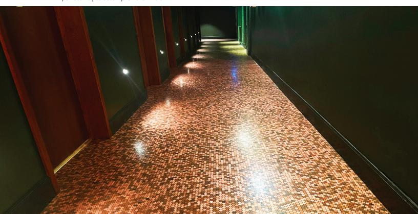
The crews began by building up the restaurant's existing bare concrete substrate with Stonclad GS, a troweled epoxy mortar system. This allowed for a cleaner transition between the tiled bathrooms and the new corridor flooring. Next came the herculean task of laying approximately 145,000 U.S. currency pennies across 419 sq. ft. of canvas in the eatery's hallway corridors.
